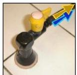
If the tap and the tube or pipe are both lined up and pointing in the same direction, then gas can flow through the tap. In other words, the tap is on.
